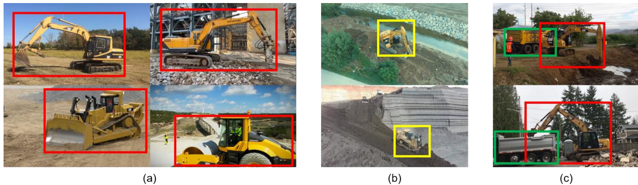
Figure 3: Example images of detected equipment by object detection: (a) positive section clips; (b) excluded section clips due to box size condition, and (c) section clips with multiple equipment detected.
