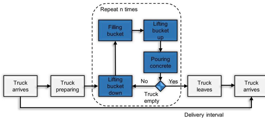
Figure 2: Work process pattern for concrete works.
