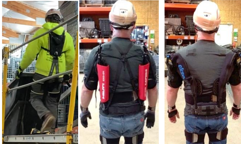
Figure 2: Three exoskeletons for tests: HeroWear Apex (Left), Hilti EXO-01 (Center), and Ekso EVO (Right). The subject also wears a full suite of sensors (e.g., in t-shirt pouches, on wrists, etc.).
