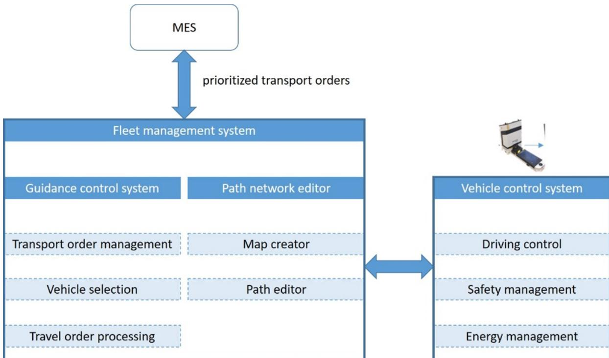
Figure 2: Tasks and functions of the AGVS.
