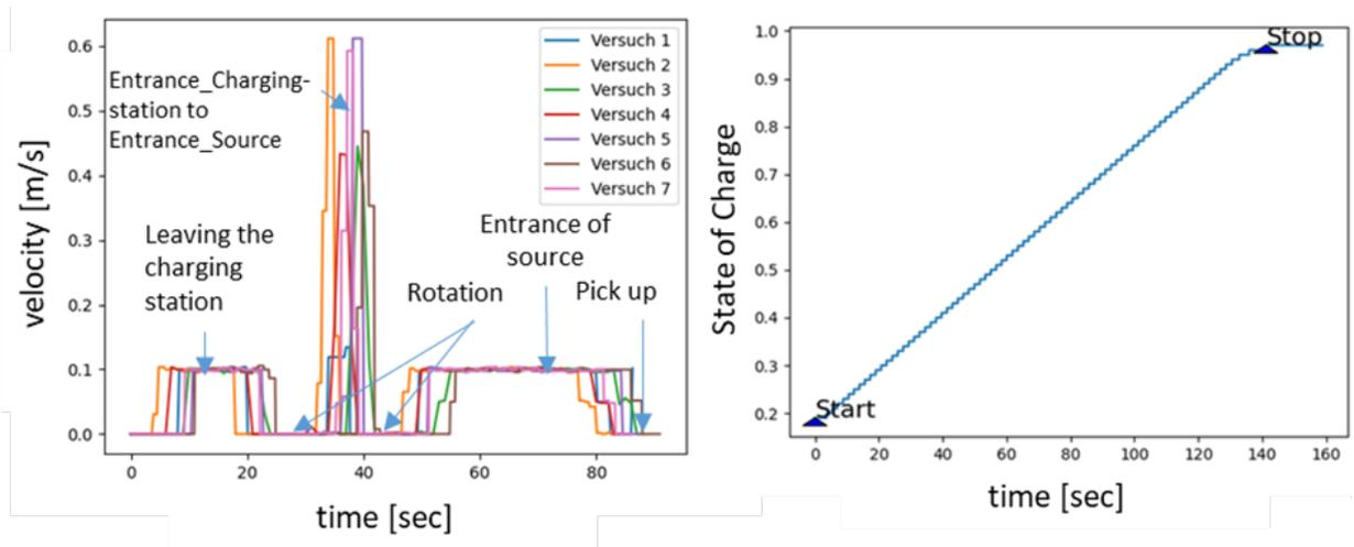
Figure 3: Visualization of real-time vehicle data: Speed profiles for various route sections (left), state of charge (right).
