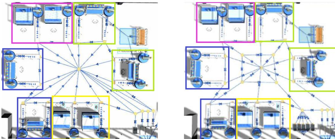
Figure 8: Star (left) and spider web network topologies (right) for the hybrid flow shop preassembly.
