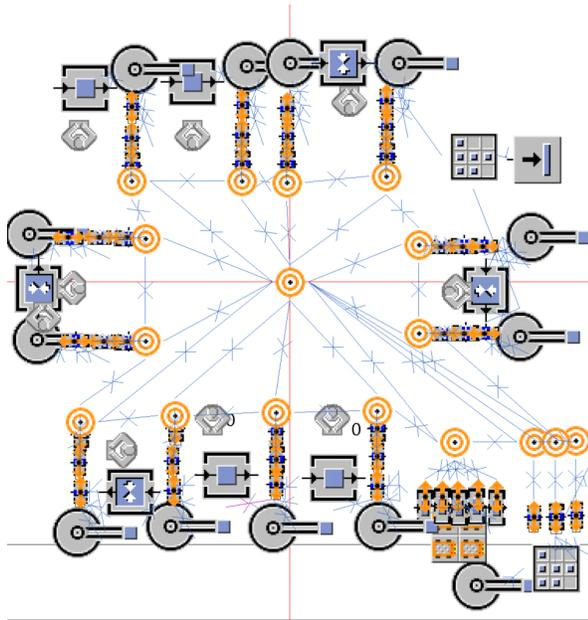
Figure 5: Routes generated by path network generator.
