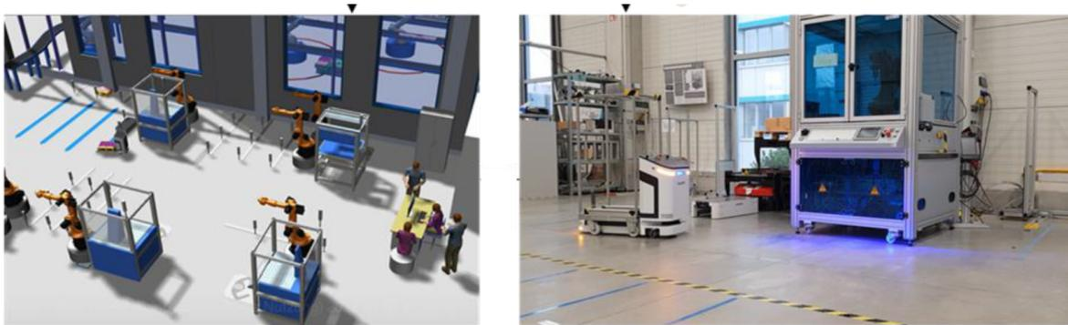
Figure 1: Use case scenario as Digital Twin simulation model (left) and real shopfloor (right).
