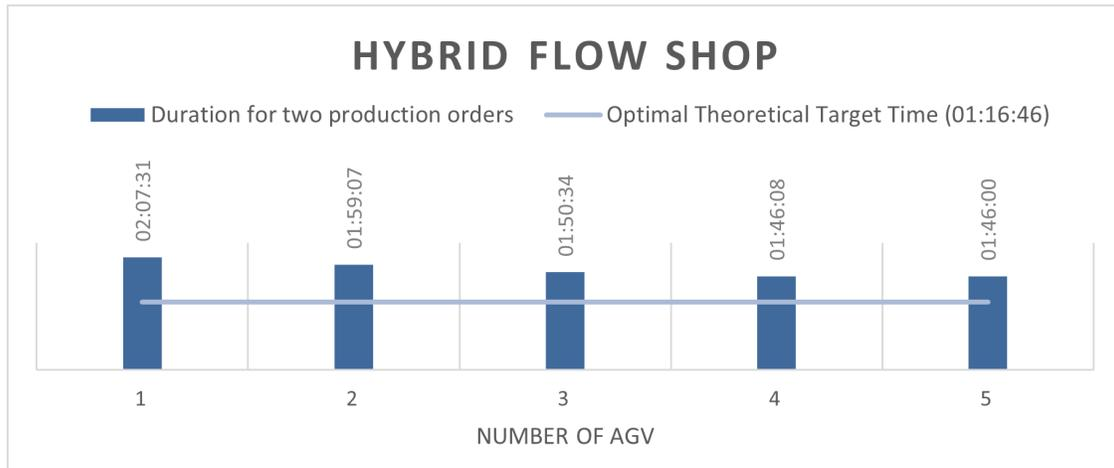
Figure 7: Throughput times with different numbers of AGVs used.
