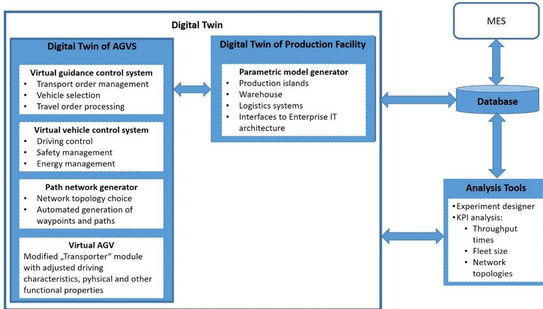
Figure 6: Interfaces of the DT with Enterprise IT architecture.
