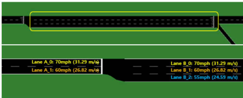
Figure 1: Roadway layout on merging zone, highlighted in yellow with speed by lane.
