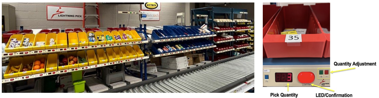
Figure 1: Example of a PTL system. A three zone PTL system (left) containing bins from which specified quantities of SKUs can be picked. Each bin location (right) has a pick quantity display, lighted pick/confirmation button, and quantity adjustment buttons.
