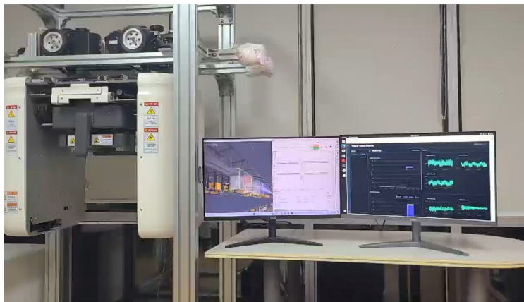
Figure 6: Virtual commissioning for an OHT system.
