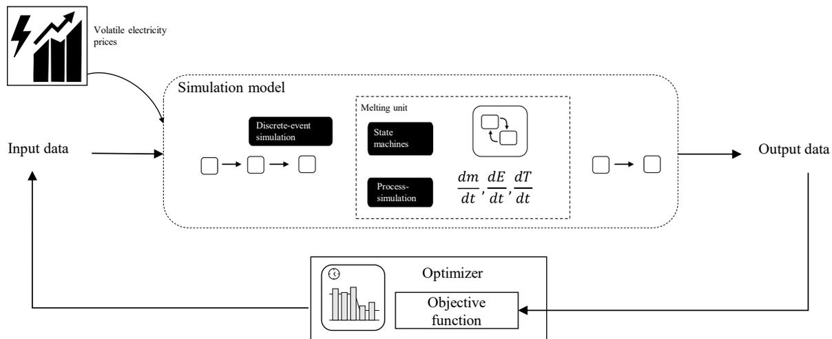
Figure 1: Simulation-based concept for the energy flexibilization of melting plants
