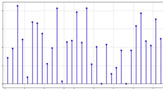
Fig. 1. Comparison between baseline and agent results. The x-axis shows the shift number (2 per day), the y-axis the percentage improvement of numbers of wafers processed by the bottleneck tools.
