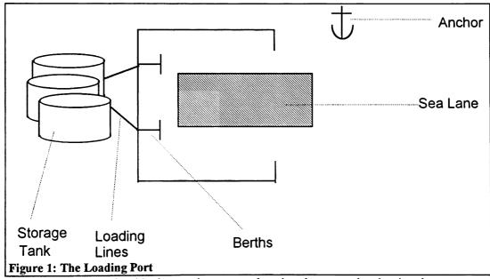
ments comprising a typical port. Outside the port is an anchorage point, at which the vessels will wait until given permission to enter. Between the anchor and the berths there is the sea lane. Usually only one ship can be moving on the sea lane at any time. In one of our simulations, this is made more complicated as there are four legs to the sea lane, different for in-coming and out-going vessels.
